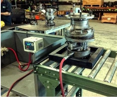
After the reman final drive motors are finished, they go to quality control. There they undergo pneumatic leak detection, calibration inspection, and hydraulic performance testing. The hydraulic performance testing includes RPM performance, brake engage and release pressure, lead test, idle test, case drain flow, and dual-speed performance (for two-speed final
