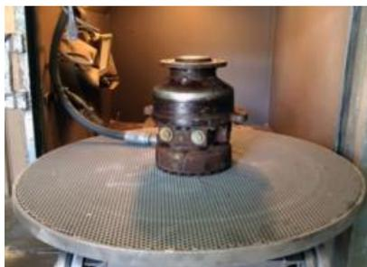
Before opening the final drive core, it will undergo sandblasting as the last cleaning step. The exterior of the final drive motor will be bare metal with no scaling, grease, or paint remaining. Only then is the final drive motor opened up.
