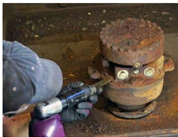
Once the core is in our system, we prepare it for disassembly. Final drives are usually covered in hardened material built up over time. This hardened material includes dried mud, clay, and other debris from a typical worksite. We use a needle scaler to remove the bulk of this material.
